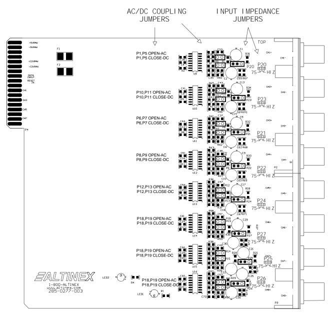
Note: In the diagram above, the jumpers are set for 75 ohms input impedance on the following ports: P20, P23, P21, P22, P24, P27, P25 and P26. (Jumpered pins have dark circles.)
